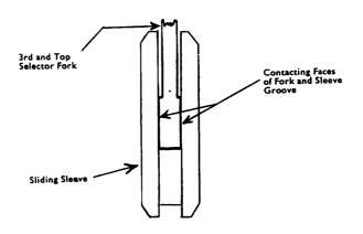
increased width of the selector fork necessitates an increase in the width of the sliding sleeve groove, and the fork and sleeve are only interchangeable with the previous type in pairs.
