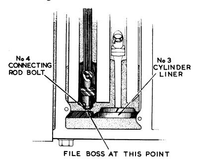
When fitting the new type connecting rods (Part No.54024) to vehicles prior to Engine No. EO/PB/10506 it is MOST IMPORTANT to ensure that there is adequate clearance between the
