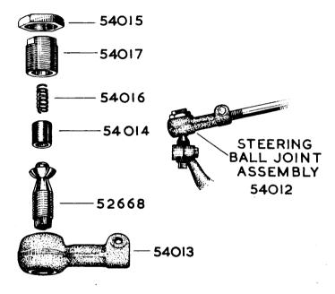
The new assembly has been designed for ease of dismantling and is fully interchangeable with the previous type of steering ball joint assembly, (Part No.52668).
