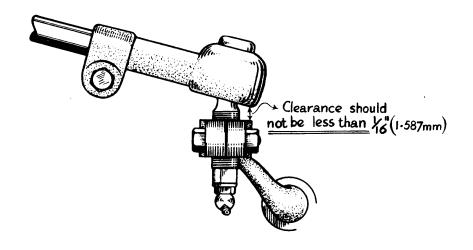
It should be noted that steering arms, part Nos. 52667 (RH) and 52666 (LH) are fitted to Right Hand drive cars and steering arms part No.52678 (LH) and 52679 (RH) fitted to Left Hand drive cars. The difference in Right and Left Hand drive models is in the height of the forward end of the steering arm in relation to the stub axle, and it will therefore be readily understood that the fitting of the incorrect arm will seriously affect the steering geometry.
